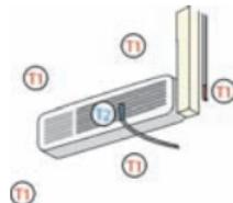
Position the hot thermistor sensor (red) ① in a suitable location at ambient air temperature. It is recommended that ceiling voids are avoided as these are usually at much higher temperatures. Place the cold thermistor sensor (blue) ② in the path of the air flow from the air conditioning unit.
