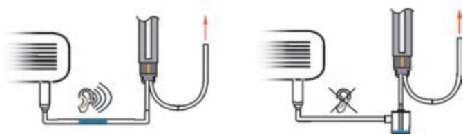
If the pump is installed remotely, occasionally water can become trapped in the u-bend at the lowest point of the system. Due to the pump's high flow rate, this can create a gurgling noise.
