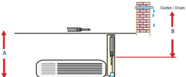
Leave sufficient space around the pump unit to allow for cooling. Ensure that the pump is not more than A above the condensate outlet, and not more than B below the desired drainage point for the pump outlet. The pump can be mounted in any orientation but must be kept DRY. (See table above for A & B). Connect the discharge tube of the pump to a suitable drainage system. Secure with cable ties where necessary. A stepped adaptor is supplied to convert various tube diameters.
