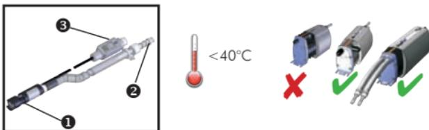
Insert the sensor ① into the condensate tray pipe as shown and secure the hose ② in position. The DrainStik™ must be mounted vertically. Use the silicon hose provided.
