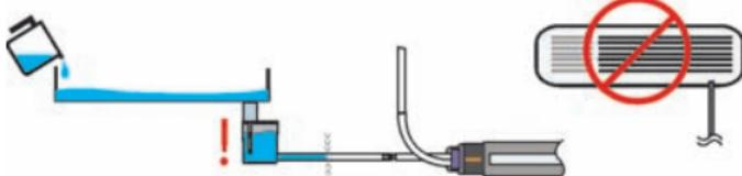
To ensure that the alarm connection is working, restrict the outlet of the reservoir/DrainStik™ hose and fill with water up to the high level sensor. The pump will turn on initially, then after a short delay the alarm relay will switch, detected using a multimeter or observing the shut down of the AC unit. Allow the water to exit the reservoir; the water should then be pumped away, and AC operation will restart.
